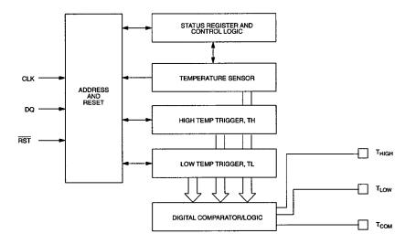
The DS1620 measures temperature using a bandgap-based temperature sensor. The temperature reading is provided in a 9-bit, two's complement reading by issuing a READ TEMPERATURE command. The data is transmitted serially through the 3-wire serial interface, LSB first. The DS1620 can measure temperature over the range of -55°C to +125°C in 0.5°C increments. For Fahrenheit usage, a lookup table or conversion factor must be used. www.trimmer.ru
